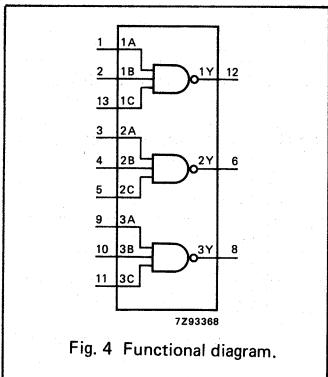
Fig. 4 Functional diagram.
