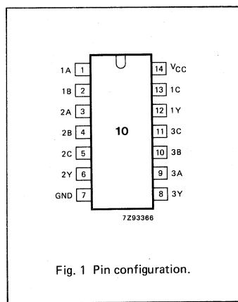
Fig. 1 Pin configuration.
