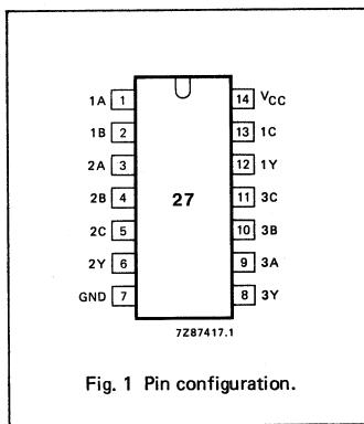
Fig. 1 Pin configuration.
