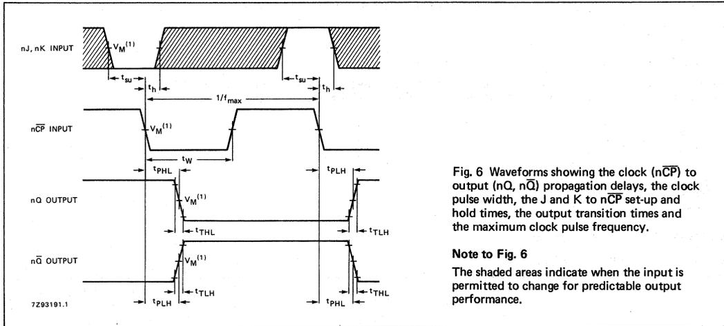
Fig. 6 Waveforms showing the clock ( $\overline{nCP}$ ) to output ( $nQ$ ,  $\overline{nQ}$ ) propagation delays, the clock pulse width, the J and K to  $\overline{nCP}$  set-up and hold times, the output transition times and the maximum clock pulse frequency.
