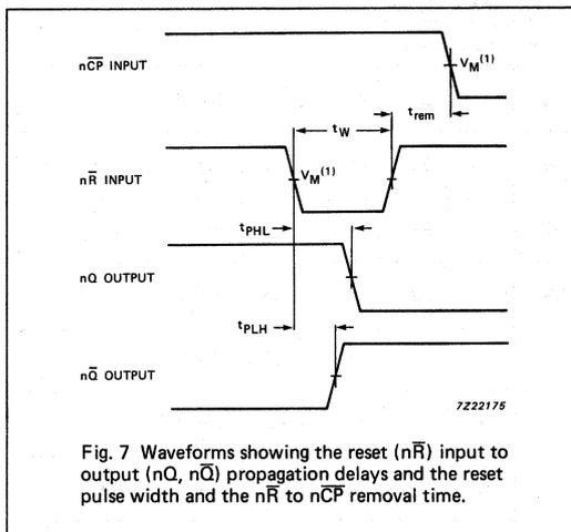
Fig. 7 Waveforms showing the reset ( $\overline{nR}$ ) input to output ( $nQ$ ,  $\overline{nQ}$ ) propagation delays and the reset pulse width and the  $\overline{nR}$  to  $\overline{nCP}$  removal time.
