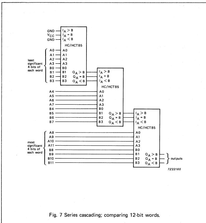
Fig. 7 Series cascading; comparing 12-bit words.
