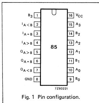
Fig. 1 Pin configuration.
