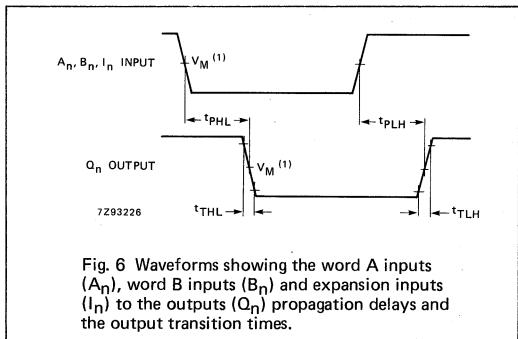
Fig. 6 Waveforms showing the word A inputs ( $A_n$ ), word B inputs ( $B_n$ ) and expansion inputs ( $I_n$ ) to the outputs ( $Q_n$ ) propagation delays and the output transition times.
