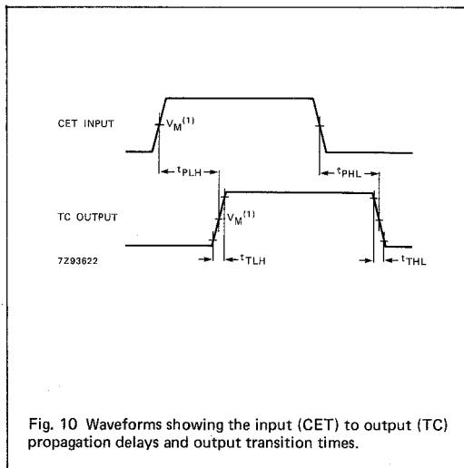
Fig. 10 Waveforms showing the input (CET) to output (TC) propagation delays and output transition times.
