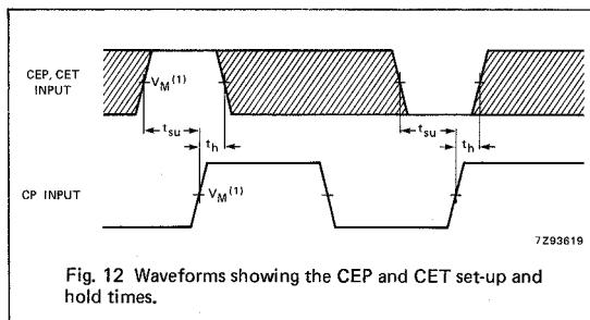
Fig. 12 Waveforms showing the CEP and CET set-up and hold times.
