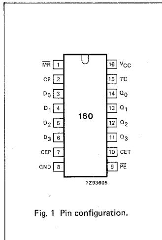
Fig. 1 Pin configuration.
