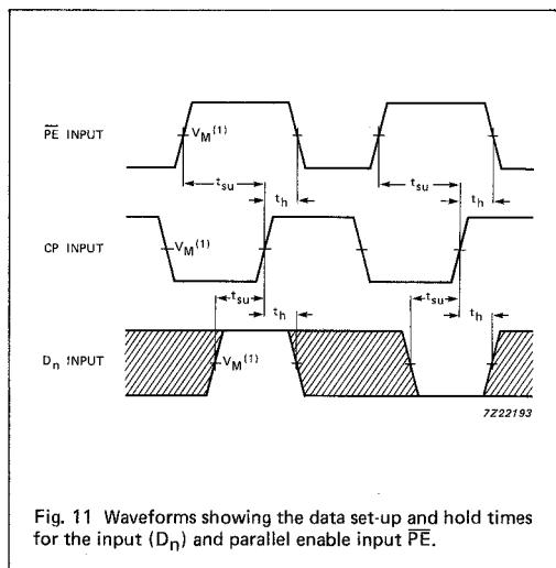
Fig. 11 Waveforms showing the data set-up and hold times for the input ( $D_n$ ) and parallel enable input  $\bar{P}E$ .
