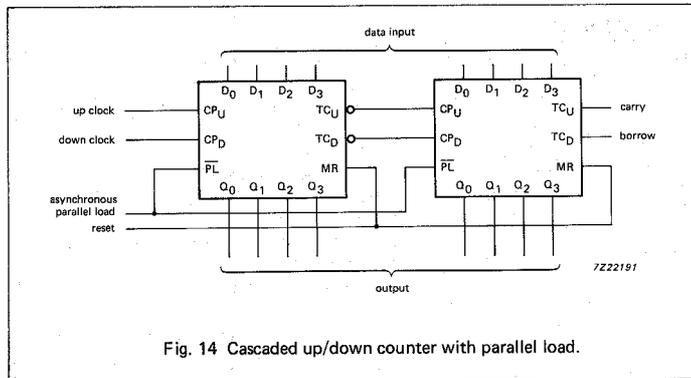
Fig. 14 Cascaded up/down counter with parallel load.
