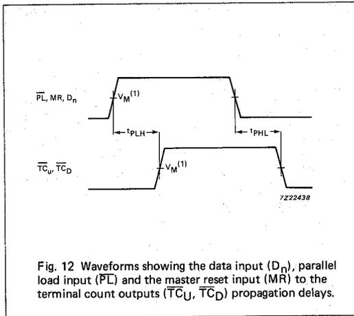
Fig. 12 Waveforms showing the data input ( $D_n$ ), parallel load input ( $\overline{PL}$ ), and the master reset input ( $\overline{MR}$ ) to the terminal count outputs ( $\overline{TC}_U, \overline{TC}_D$ ) propagation delays.
