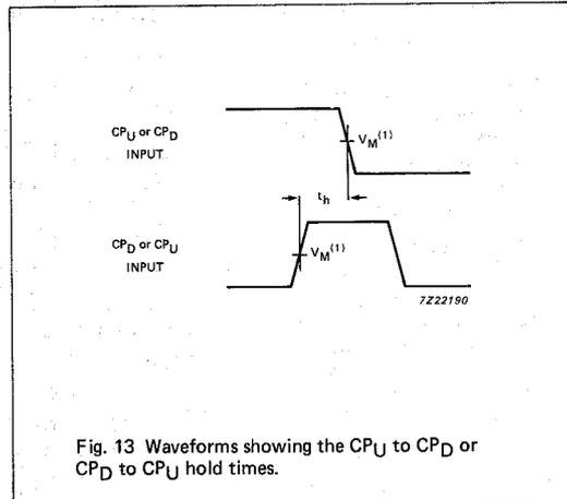
Fig. 13 Waveforms showing the  $CP_U$  to  $CP_D$  or  $CP_D$  to  $CP_U$  hold times.
