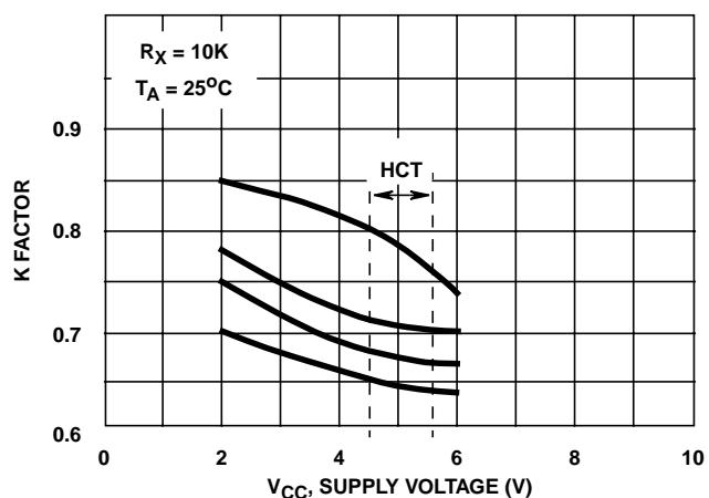
FIGURE 6. HC/HCT221 K FACTOR vs SUPPLY VOLTAGE
