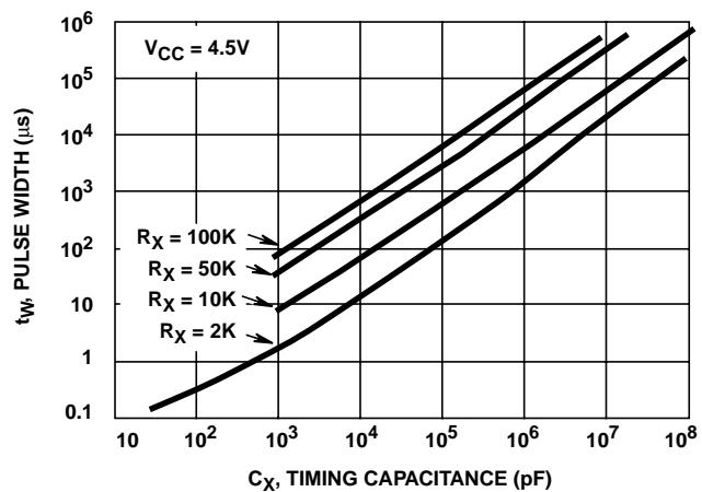
FIGURE 8. HC/HCT221 OUTPUT PULSE WIDTH vs  $C_X$
