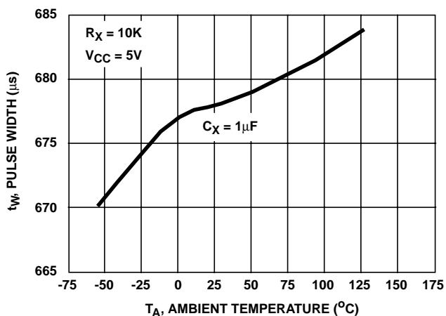
FIGURE 5. HC/HCT221 OUTPUT PULSE WIDTH vs TEMPERATURE
