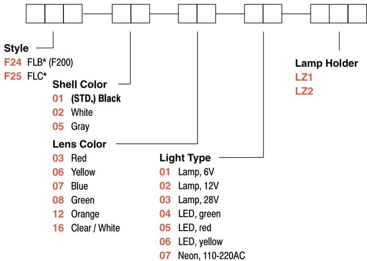
\*Button options for central mounting configurations, use 'FG' for central mount with chrome dress nut, use 'FA200', 'FLB' or 'FLC' for central mount with black dress nut.
